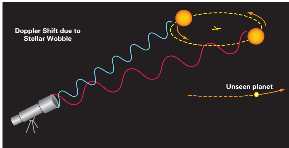
FIGURE 2-16 The technique used by several teams of scientists to detect planets around Sun-like stars by searching for periodically changing Doppler shifts in the stars' spectra. The diagram shows a particular star at two positions in its orbit. The successive redshifts and blueshifts of that star's spectrum reveal the otherwise unseen planet. It must always be on the opposite side of the system's "center of mass" (like the fulcrum of a see-saw; Chapter 11 has more details) from the star.
